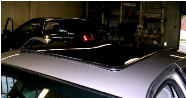
A test fit. Note the distance between the corner of the sunroof frame and the CV's top. While side to side curvature is no problem, the front-to-back curve of the roof leaves a quarter inch or slightly more gap on the corners.
