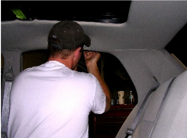
Tracy begins tucking the headliner material under the original headliner and attaches trim such as the B and C pillar interior panels, rear grab handles, etc.
