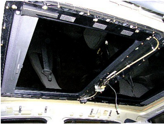
The sunroof module is set in place for a final fit.
