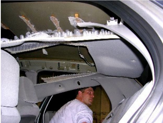
Note the bubble insulation between headliner and roof.
