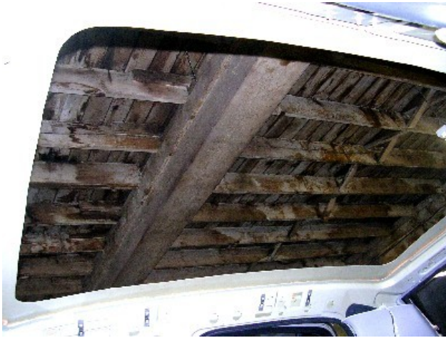
The opening is roughed in. (That's the ceiling of Rose City Sunroofs as seen through the new hole in the CV's top.)
