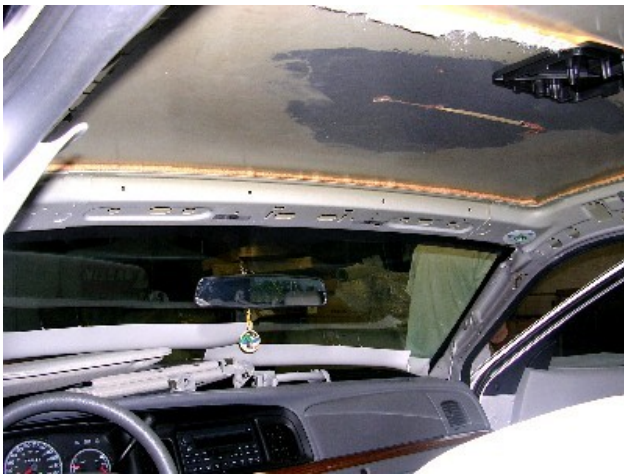
The CV roof has no cross members. Roof support comes from the perimeter structure.
