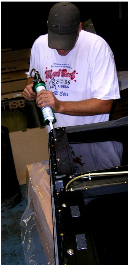
After test fitting three times and adjusting the CV's roof hole, it's time to silicone seal the module.
