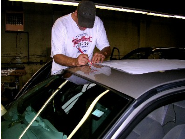
Using a grease pencil, Tracy outlines the pattern onto the roof.
