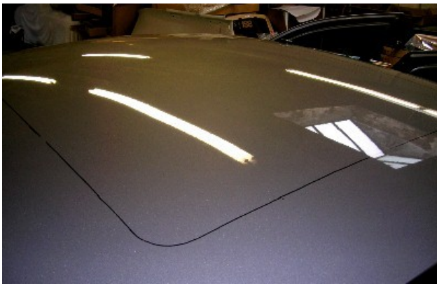
The marked area to be cut.
