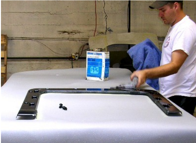
The front headliner frame is cleaned.
