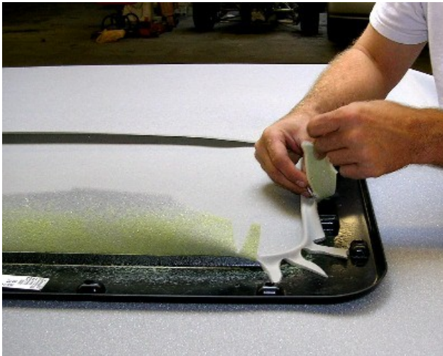
Headliner material is glued to the inside edges and corners, but not to the top (underside here) to avoid bunching or “fingerprints” when installed.
