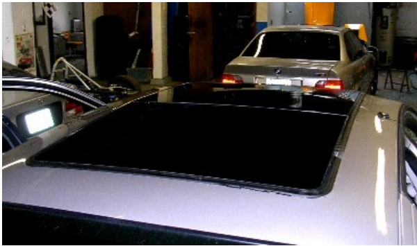
The top installed. You can still see the silicone residue on the roof which Tracy removes with a razor blade with the cardboard cover still on.
