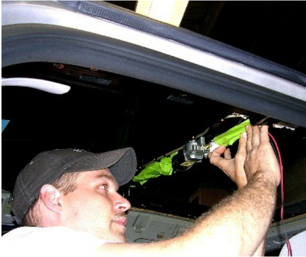
Using strong tape and the fuzzy side of Velcro as a wrap, Tracy assures a rattle free installation.
