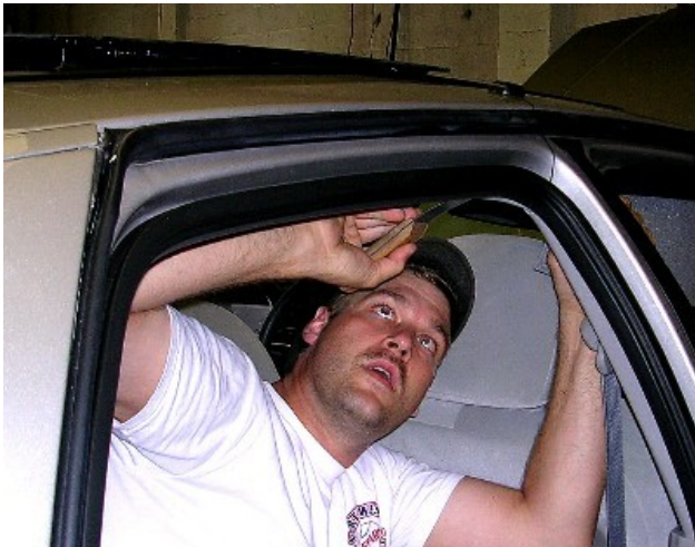
More work on the headliner using what looks like a putty knife.
