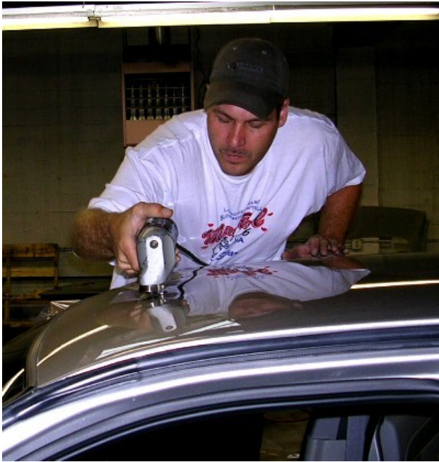
He then begins cutting the opening following the grease line.
