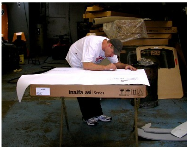
Tracy cuts out the sunroof-frame pattern using a razor blade.
