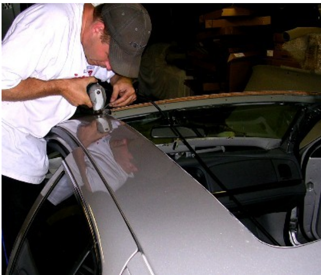
Tracy trims the corners of the hole to give the frame a bit of breathing room.
