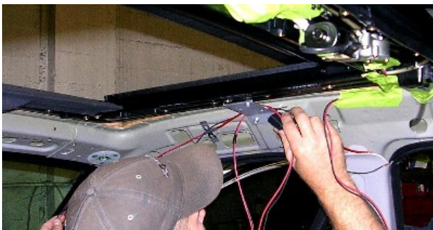
Sunroof wires are strung...
