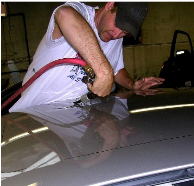
Let the cutting begin. Tracy makes a hole in the roof which turns into a “handle” for lifting out the metal.
